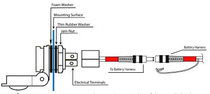
Accessory sockets require 1.75 inches of clearance behind mounting panel. DO NOT use a flat wood drill bit, this will elongate the hole.
